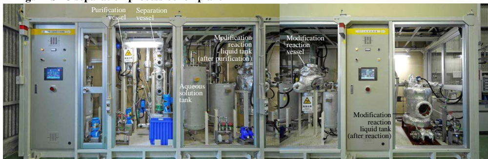
Fig.10 SFC modification process bench plant
